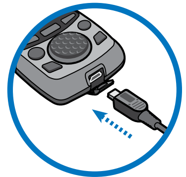
Fig. 3: Inserting the mini-USB connector
